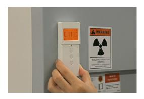
Options: Nuclear radiation detector  $\label{eq:multifunctional} \mbox{Multifunctional ray detection, including } \beta, \mbox{X-ray, } \gamma \mbox{-ray detection,} \\ \mbox{Rechargeable design greatly improves battery life, fast test} \\ \mbox{speed, increased CPM display and automatic range, wider} \\ \mbox{measurement range, built-in filter function, to avoid other} \\ \mbox{interference}$
